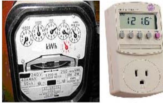
Figure 5.4 Measurement of Power
